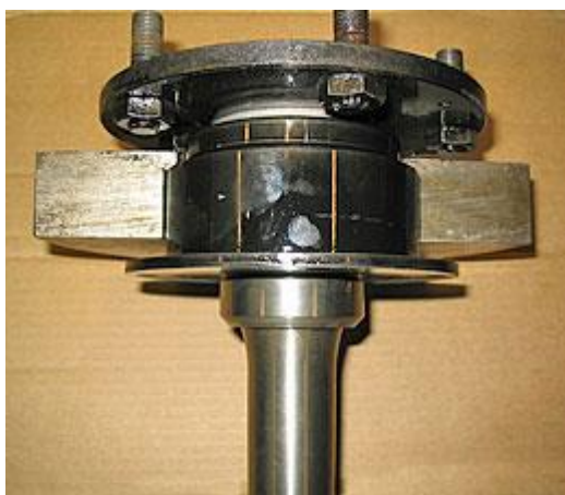
Supporting block showing how the block lip embraces the bearing housing
