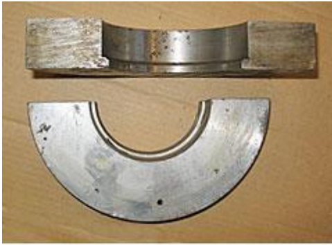
Supporting blocks showing shape to support the bearing housing
