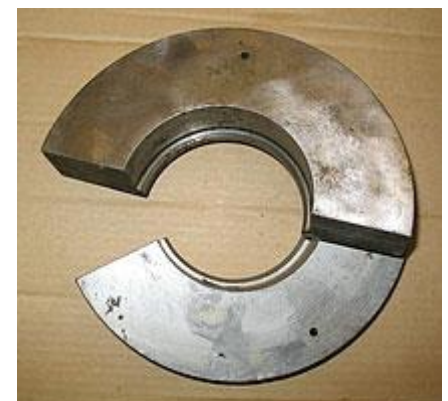
Supporting blocks to hold the bearing housing during pressing operations
