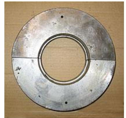
Supporting blocks showing how they surround the bearing housing
