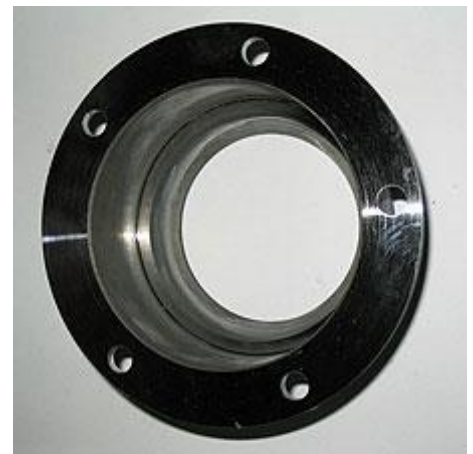
A wheel bearing housing after machining and the flange has been ground
