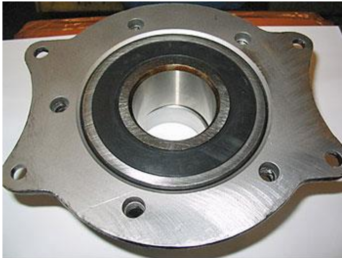
Fig 12. The bearing housing after pressing in a 3309 2RS bearing
