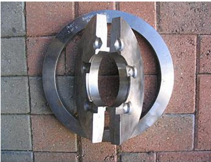
Fig 5. Hub support tool showing the split joint
