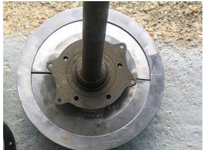
Fig 8. Hub support tool assembled onto an old half shaft, note the outer ring
