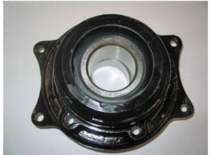
Fig 13. The opposite side of the bearing housing fitted with a 3309 2RS bearing
