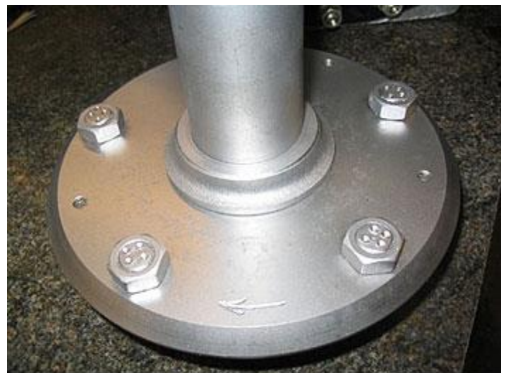
Fig 10. The half shaft with the spacer fitted, ready to accept the bearing assembly
