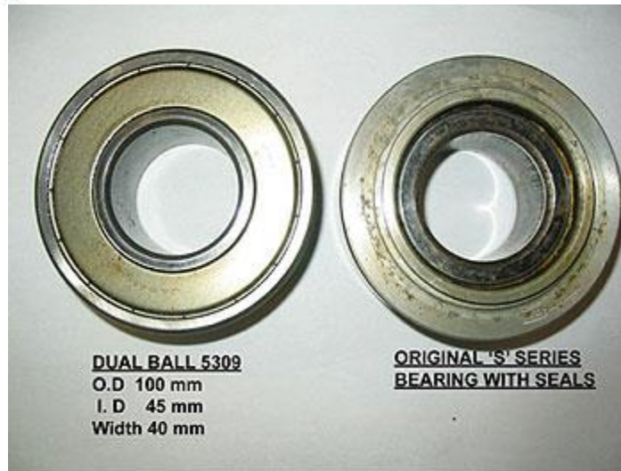
Fig 4. Side view of a 5309 and an original S type bearing including oil seals
