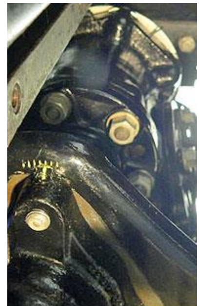
Picture 4. Vernier adjustment on steering box 1
