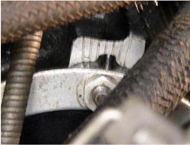
Picture 3. Uppermost steering box adjustment
