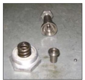
were made of fairly soft brass and after 50 years tended to be glued to the tie rod end
