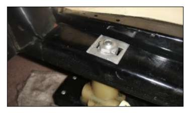
At left is the mount for the top of the jack. The screw shaft is very firmly anchored in the two securing plates to prevent its turning during jacking. The seat here is at maximum height.
