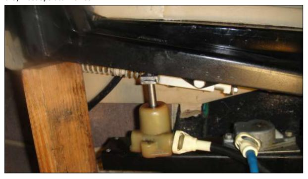
The blue flexible cable, one of two, drives the gearbox that traverses the seat fore and aft.
