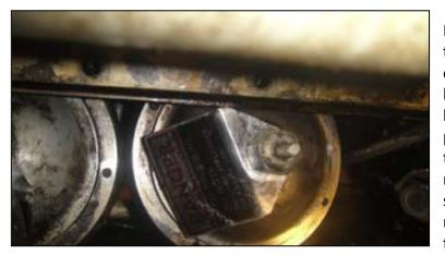
By now we have all appreciated that a couple of small canisters of high pressure nitrogen stands between the average driver and his Maker! Brake fluid is pumped into these spheres up to about 2,600 psi when the regulating valves sitting out of sight here on top of the spheres redirect the pump output back to the reservoirs. We all also
