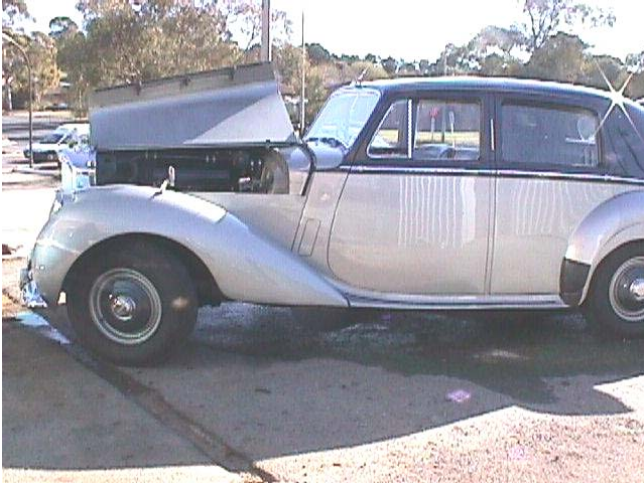
John Beagle's Bentley cocked a leg on the nearest curb so that John could adjust the drag link rebound dimension.
