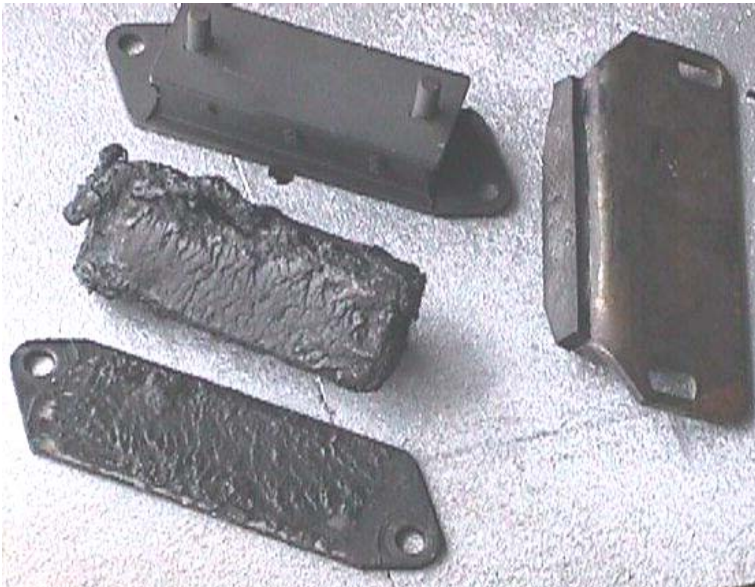
The new Mount at top the delaminated one beneath, the stop plate with a new bit of rubber at right
