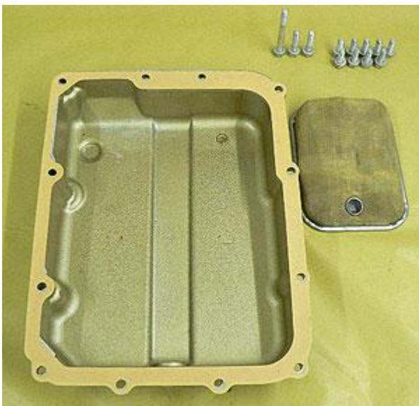
The sump and clean fluid filter from my transmission. Cleanliness is vital if reliability is to be preserved.
