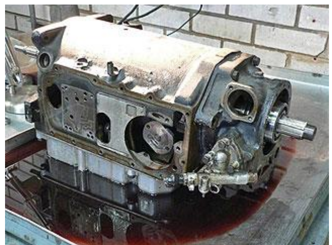
This is a view of a partially dismantled Bentley R type transmission. The different tailshaft housing and ride control pump can be seen.
