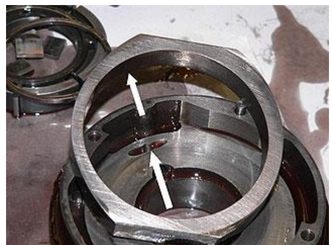
The pump body and oil control ring. The torus oil feed may be seen arrowed in the pump body. The spring loaded oil control ring covers this oil feed port when the torus is full of fluid. If the pump has been re-machined there may be the possibility that the oil control ring is no longer able to fully cover the port in it's closed position. If this happens, full main line pressure is delivered to the torus. This causes the torus to burst its seals and causes severe leaks. Make absolutely certain your pump is perfect before installation.
