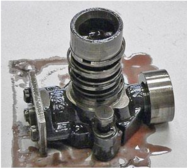
The governor assembly. Here can be seen the sealing rings. They look like piston rings sitting in their grooves at the top of the component.
