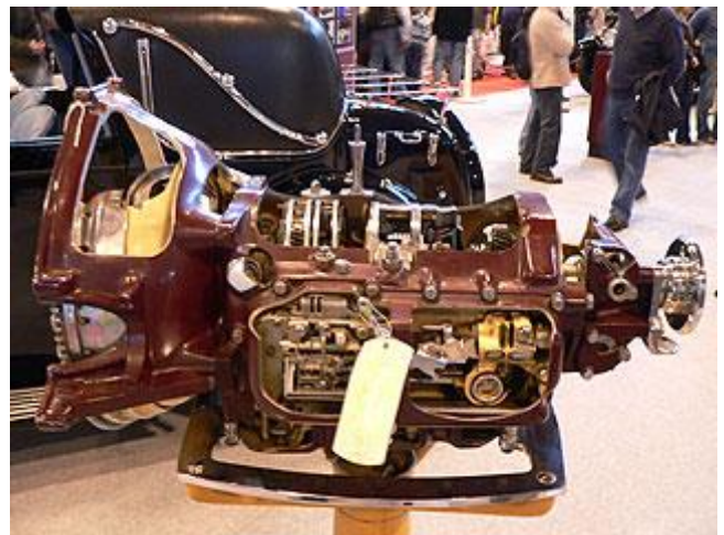
Photographs of a cut-away Rolls-Royce Hydromantic gearbox taken on a recent exhibition
