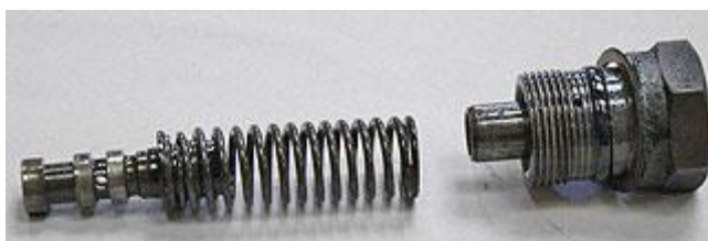
The main pressure regulation valve. This valve screws in to the top of the transmission near to the band adjusters near the bell housing. It controls the main operating pressure of the transmission. IT IS VERY IMPORTANT 6 CYLINDER VALVES ARE NOT INTERCHANGED WITH V8 VALVES. they run at different pressures, the V8 being the higher pressure.
