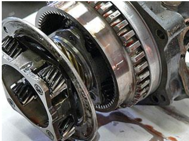
The reverse epicyclic gear cluster. Just behind it is the rear epicyclic cluster contained in it's "toothed" annulus. The annulus has teeth cut into it to engage with the locking pawl. With the car in reverse with the engine switched off the pawl engages with the rear annulus to lock the transmission.
