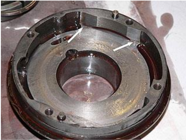
The main pump body. Problems can arise in the areas arrowed. It is impossible to machine into the corners of the casting. If the excess metal is not relieved from these areas with a rotary file or similar, the rotor can pick up causing the pump to seize.
