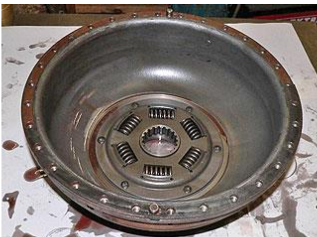
The torus cover. Note the antishock damper springs in the centre, and the opposing locating pins in the outer mating face. The smaller pin is usually located near the torus drain plug
