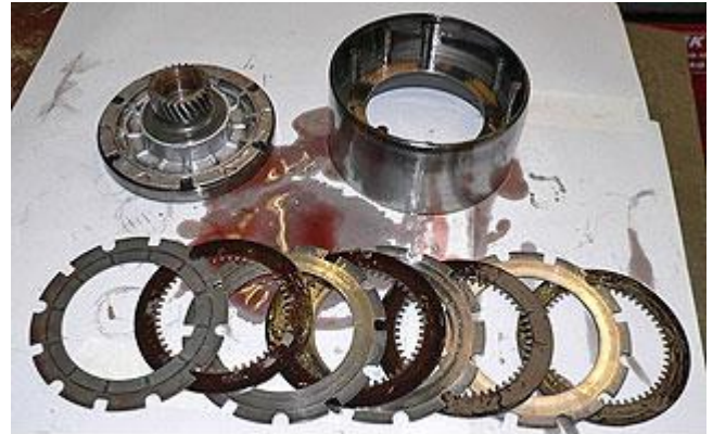
The front brake drum is shown to the top left. To the top right is shown the front sun gear from the front epicyclic gear train. The lower part of the picture shows the front clutch plates.
