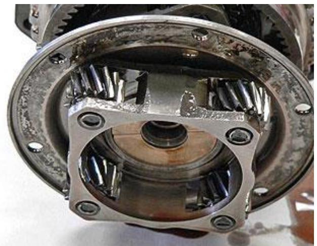
The rear forward drive epicyclic gear train with one of the bronze adjusting washer in the centre. The reverse epicyclic gears and the locking annulus can be just seen behind.
