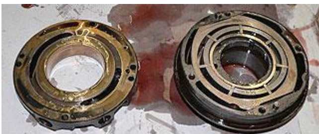
The main pump. To the left is shown the main pump body complete with rotors and vanes. To the right is shown the cover.
