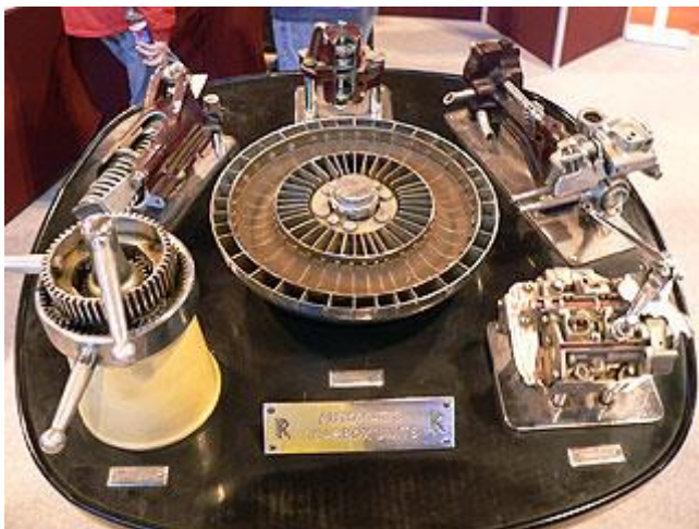
Photographs of a cut-away Rolls-Royce Hydromantic gearbox taken on a recent exhibition
