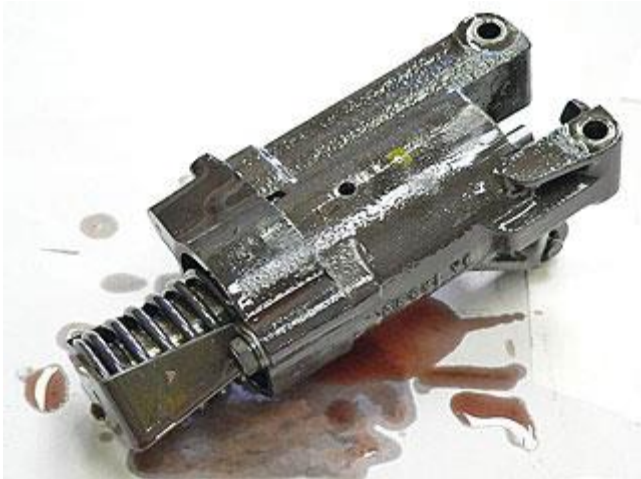
The rear brake band servo. ( A special tool is needed to dismantle and re-assemble this component)
