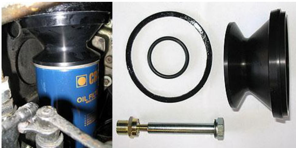
Filter and adaptor kit for R Type of MKVI with single central fixing bolt
