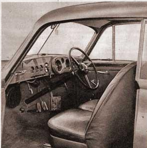
The massive fascia in polished walnut is almost entirely occupied by instrument dials and switches. Below are seen one of the heater elements, the pendant pedal for the one-shot lubrication and a fresh-air duct by the throttle.
