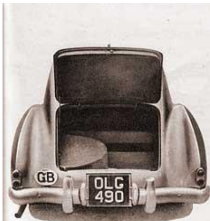
The spare wheel, which is carried on the floor of the luggage locker, has a special cover to prevent damage to the luggage. Jack and tools are carried in a special compartment below the floor of the locker.
