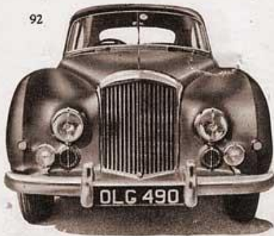
The special radiator shell is smoothly faired into the bonnet and the concave curves of the wings, to give a new and modern appearance to the Continental Bentley. There is a curved wind-screen supported in very slim pillars.
