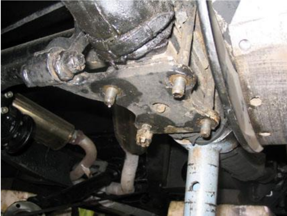
The last nut being removed on these “U” bolts
