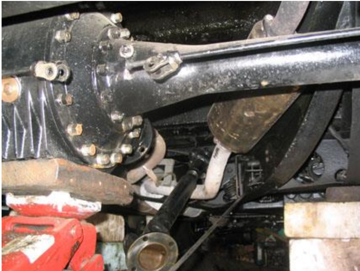
In this view the drive shaft has been disconnect and the brake equaliser removed
