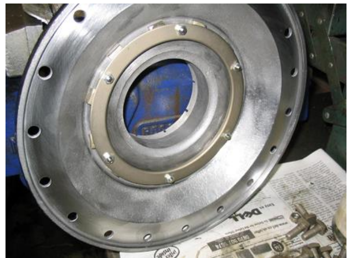
The locking plate fitted to the square bolt heads, not a sight you will see unless you are unlucky or careless
