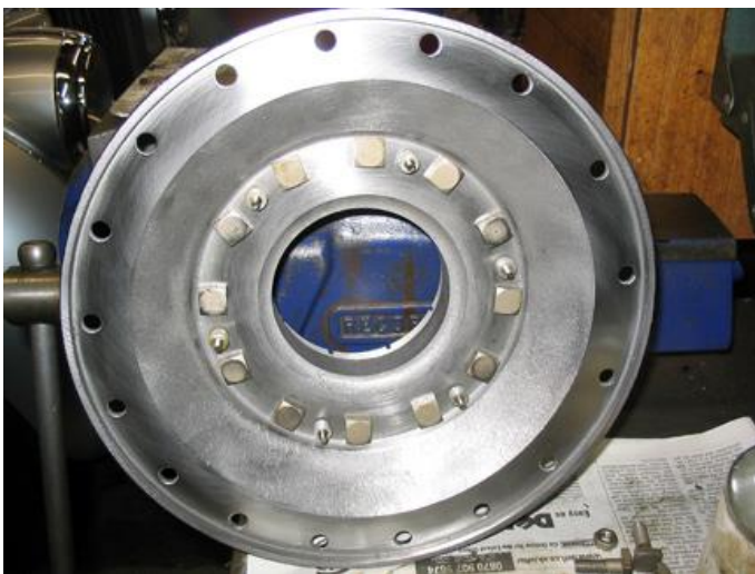
The axle side plate square headed bolts before fitting a locking plate
