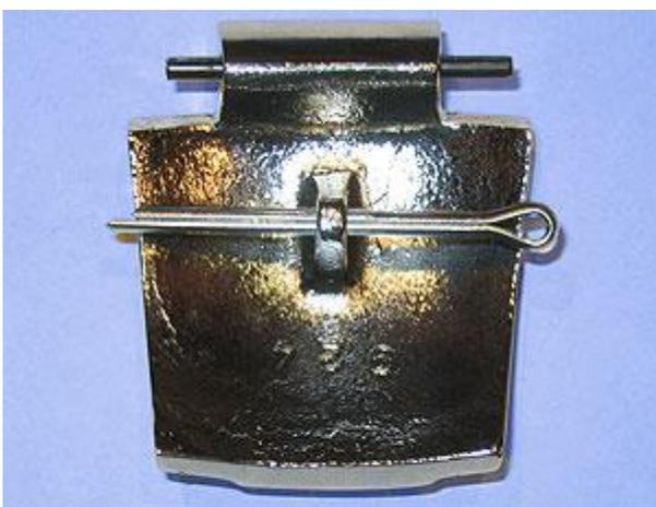
Fig C. Shows the two pins needed to attached the flap to the bodywork and toggle mechanism.
