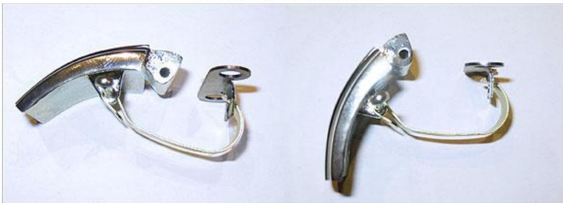
Fig F. Illustrates the assembly off the car. Left in the open position, and right in the closed position.
