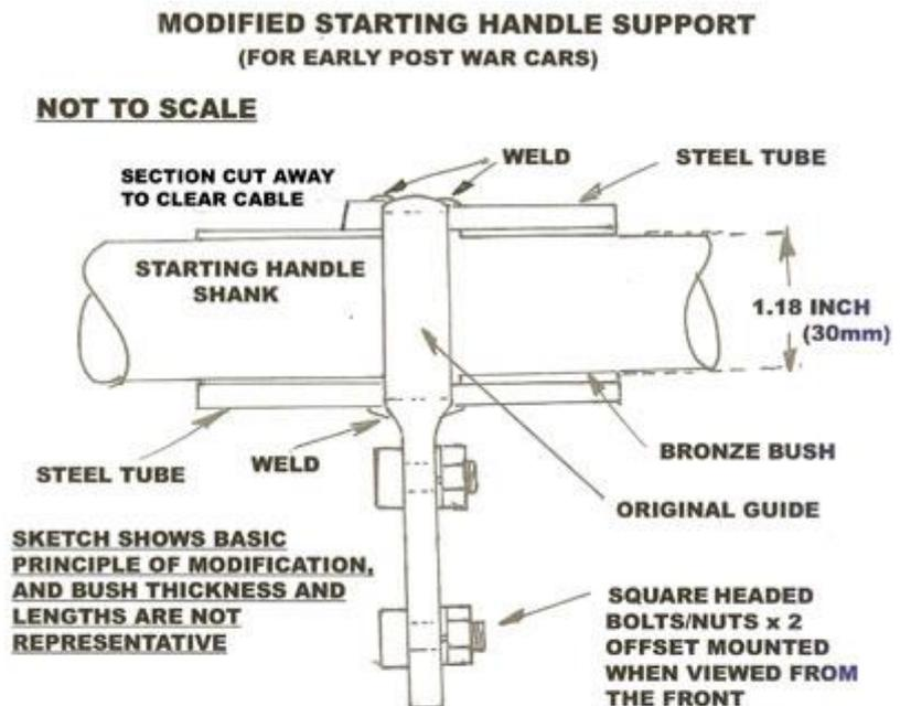
Fig H. Shows a sketch of the modified starting handle support
