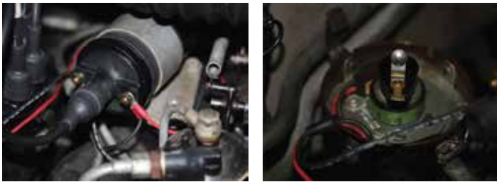
Pictures 2 and 3: Installation on Silver Cloud II: extra red wire which powers sensor is connected to Positive terminal on coil
