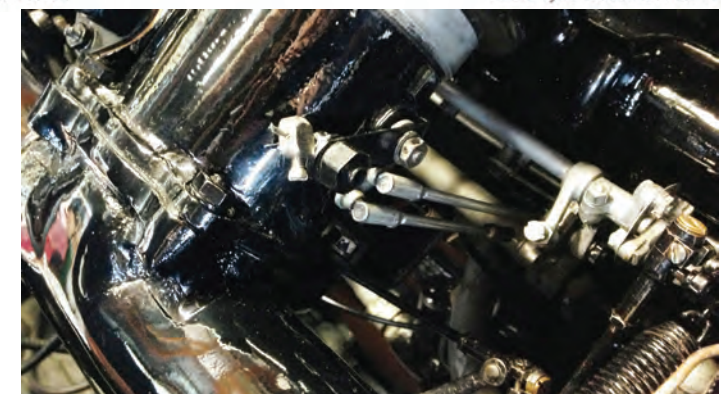
This shows the small lever (black) which operates the choke over-ride. Just visible is the hole in the bolt head where the Bowden cable is free to slide. Clamp on the cable end.
