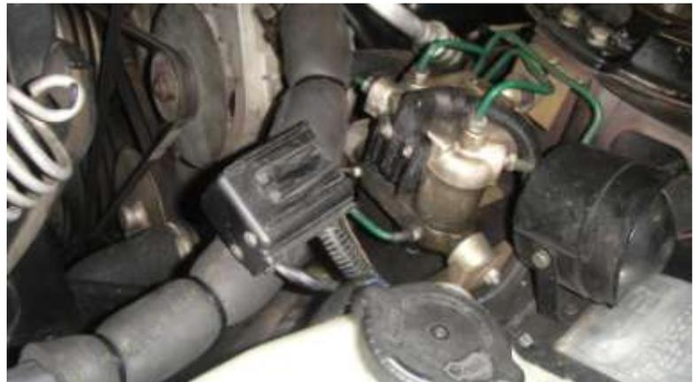
The above is the gubbins for the ABS system (antilock brake system). The small grooved box lying on the insulated air conditioning pipe should be held to the rest of the assembly but it seems that being continually smacked by the pipe
