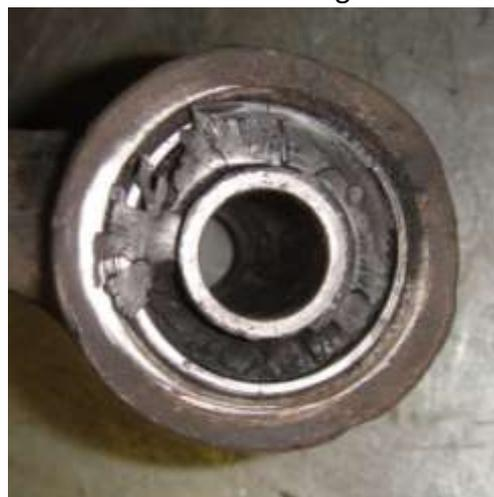
Finally I dragged out the upper suspension arm and found the source of the bocking – the silentbloc camber bush. The bright metal on the arm is where the arm has been able to move back and rub on the mount.
