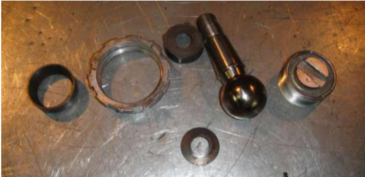
Here is the whole gubbins laid out. The adjusting cap is on the right, the friction cones are much slimmer than the lower ball joint items and the small Belleville washer sits on the top cone to help keep its shape. The slot in the adjusting cone is clearer here. My earlier reference to the product of an illicit liaison by name, applied to a bastard file. The end of a large thick example of one of these and a stout adjusting spanner are ideal for tightening down that cap.
