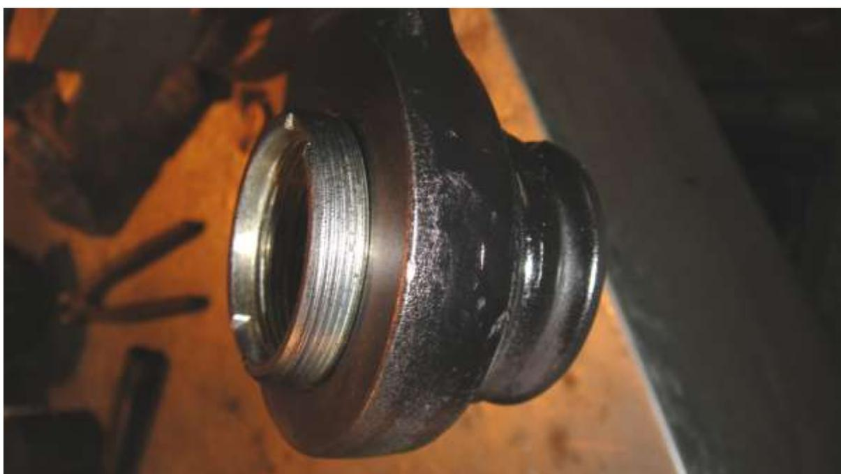
Retaining ring off, the rubber boot can be left in place if it's in good condition. Note the slots machined in the top of the bearing casing. The slots in the housing are provided to allow the adjusting cap lip to be peened at these points to lock it in place.
