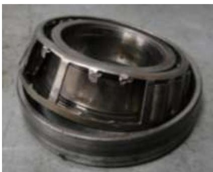
This was a nasty surprise. When I bought the car the supplier remarked that they had to fiddle with one of the front wheel bearings but it was 'all OK'!!!!!!!!!!!!!! Like the trusting idiot that I am I had not bothered to check the result of their 'fiddling'. When I pulled the front hub off this was what greeted me. Had a bit of that cage got jammed in the rollers, I may well have departed
