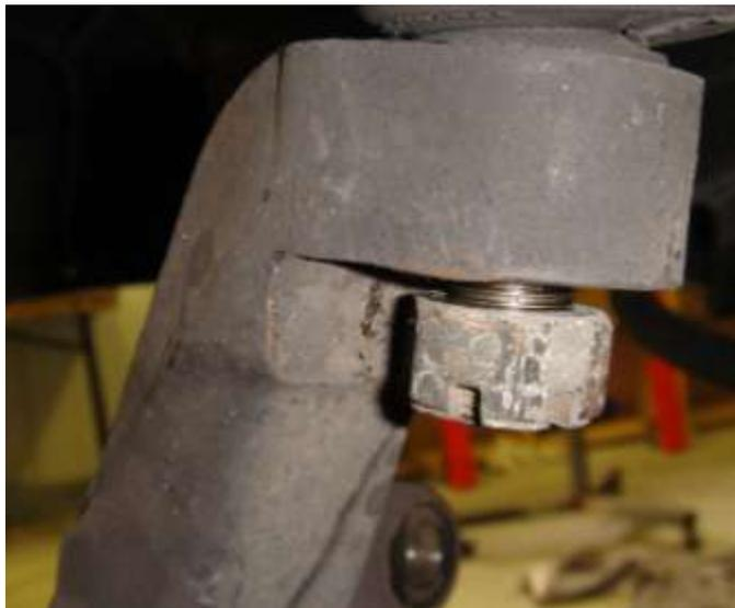
the retaining nuts about 3/16" obviously with the car on stands and the wheel unsupported. The pictures show the bottom yoke bearing above and the upper yoke bearing below. All that remains is to use a large brass drift and a brickies hammer to belt the yoke. If you find a serious attack of bursitis coming on, stop hammering and apply a little heat then a couple of bangs.
