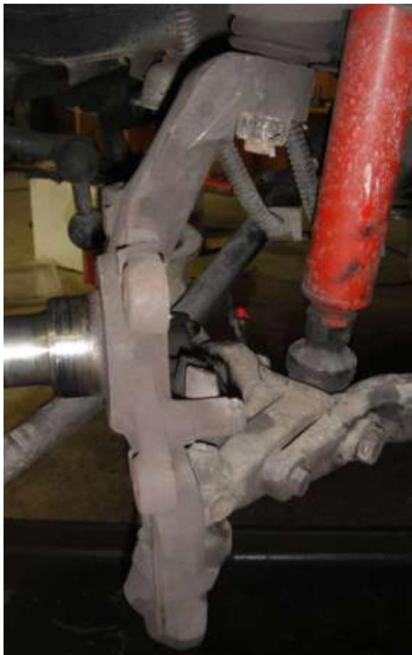
The first wheel I tackled (the right one) I simply (?) disconnected the steering arm and the brake lines. Having undone the ball joints I lifted the whole assembly and carried it to the bench, then retired to my cot to get over the strain. The assembly of rotor, two calipers and yoke is very heavy. Sense prevailed for the left side and I dismantled all the detachables before lifting!
