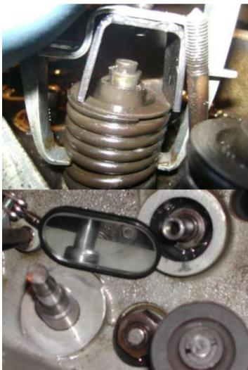
At right can be seen a locating ring that is placed over the guide which is made up to replace the original small 'top hat' since that item and its spring has no function with the new seal. The 'rim' of the discarded
