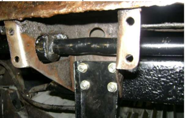
pass over the body of the unit and as can be seen below there is a suitable bump in the bar to accommodate the ram..
