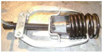
At left is the tool now used for removing valve springs. The legs that grip the coils are offset to allow for the coils and the cap is pushed down by an adjustable saddle seen here.
