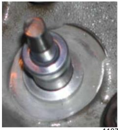
'hat' was designed to keep the larger 'hat' concentric to the valve and stop the spring slithering around on the head. The locating ring now in place does this job and keeps the large 'hat' in place. Here the new seal has been pushed over the valve stem and onto the top of the guide. This requires a thin plastic cap over the valve to avoid any damage to the seal as it crosses the sharp edges of the collet groove.
