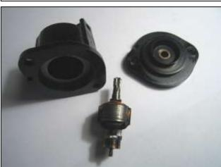
end shaft and gear. Also put a small amount of high melting point grease on the gear seen through the centre hole seen in the picture below.
