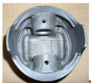
measurable wear in the bores. In the aggregate there was about a thou (.001") more clearance between the piston and the liner than desirable so the liners and pistons were shipped off, where the former were honed and the latter were Teflon coated. This was all new to me but I am assured it is the modern approach and very effective.
