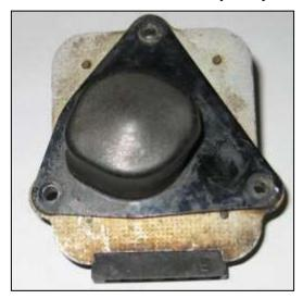
Usually all that is required is for the bearings and gears to be lubricated. This should not be attempted with the actuator in position as it is very easy to lose the very small brushes and springs.
