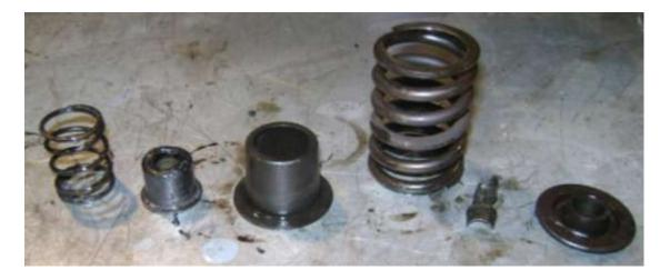
The bits above were removed from the valve in the first picture. The 'top hat' and smaller spring at the left, fit over the old seal and the top of the valve guide, these in turn are held down by the larger 'top hat' which also has the job of holding the bottom of the valve main spring in place. The last two items are the spring cap and the little collets that fit in the grove at the top of the stem which can be seen in the first picture.
