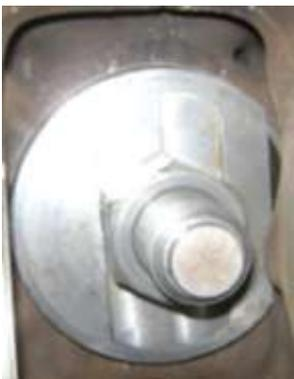
It is important that a liner is not pulled that is not supported by a block end and/or another liner! This is because the webs at the bottom of the liners are the weakest part of the casting, it is also the point where most of the detritus from the cooling system collects and sticks to the bottom of the liner. Pulling this past a seal may be just too much for the casting.
