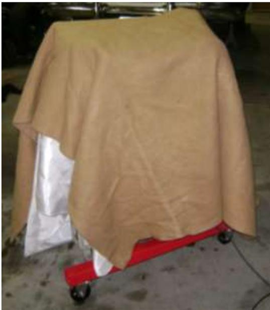
It is essential that the whole block is heated. Not having the prescribed hot air oven to raise a temperature of 150 degrees C, I settled for 80 degrees C by putting a 2,400 watt radiator under the block with a fire blanket and an old army blanket to keep the heat in. This took about 4 hours.
