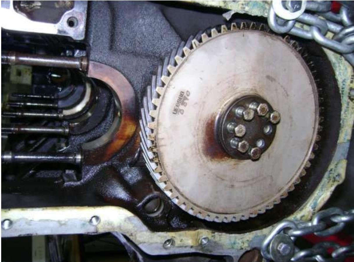
The crankshaft has been removed with the respective bearing shells and the eight bolts securing the camshaft gear are being removed. These do not have lock plates or washers under the heads. The hole near the gear on the lower side is the input point from the oil pump.
