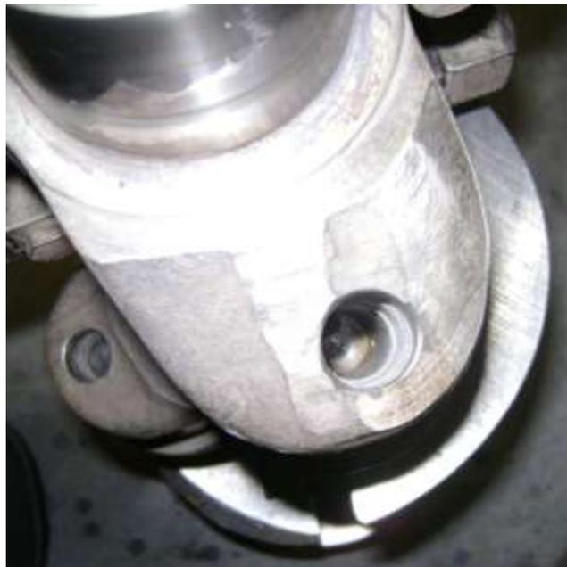
The 'plugs for the traps have a simple 'O' ring around them to keep the seal. When replacing the seal it is a good idea to replace the circlips as well – after all they have been 'accumulating' for nearly 40 years!
