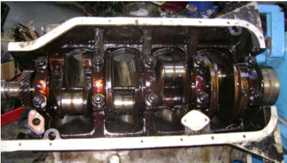
The heads are off, the oil pump removed from its mount at bottom left as has the pickup stirrup which is bolted to the crankcase on the lower side further along. I have been asked whether I will convert the sealing arrangements for the ends of the crankshaft to match the
