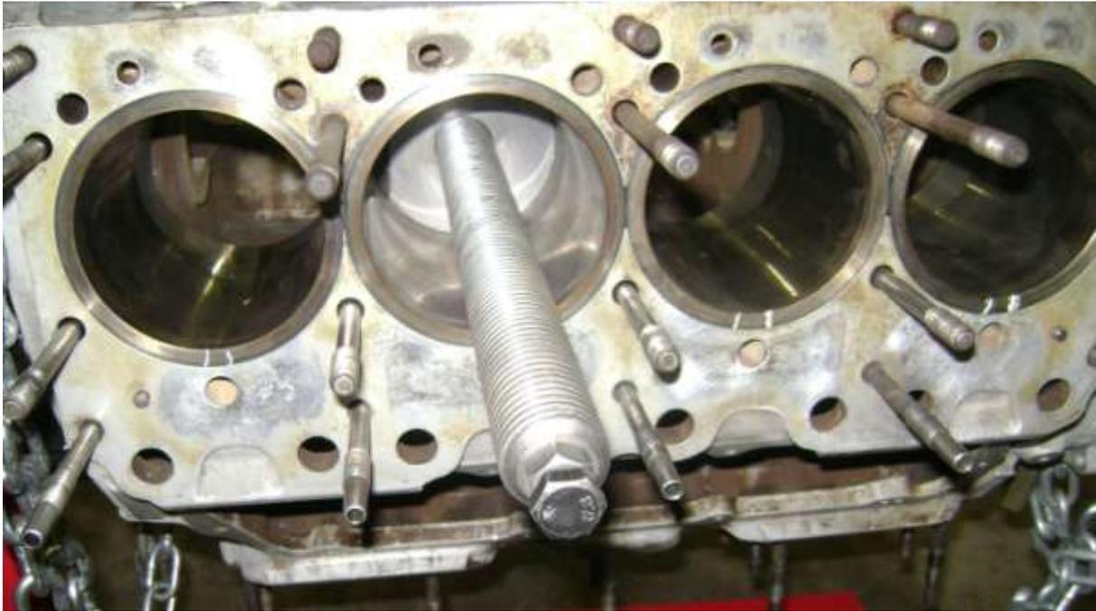
The moment of truth has arrived. The cylinder liners have to come out to clean out the water passages and replace the liner seals – all three of them.
