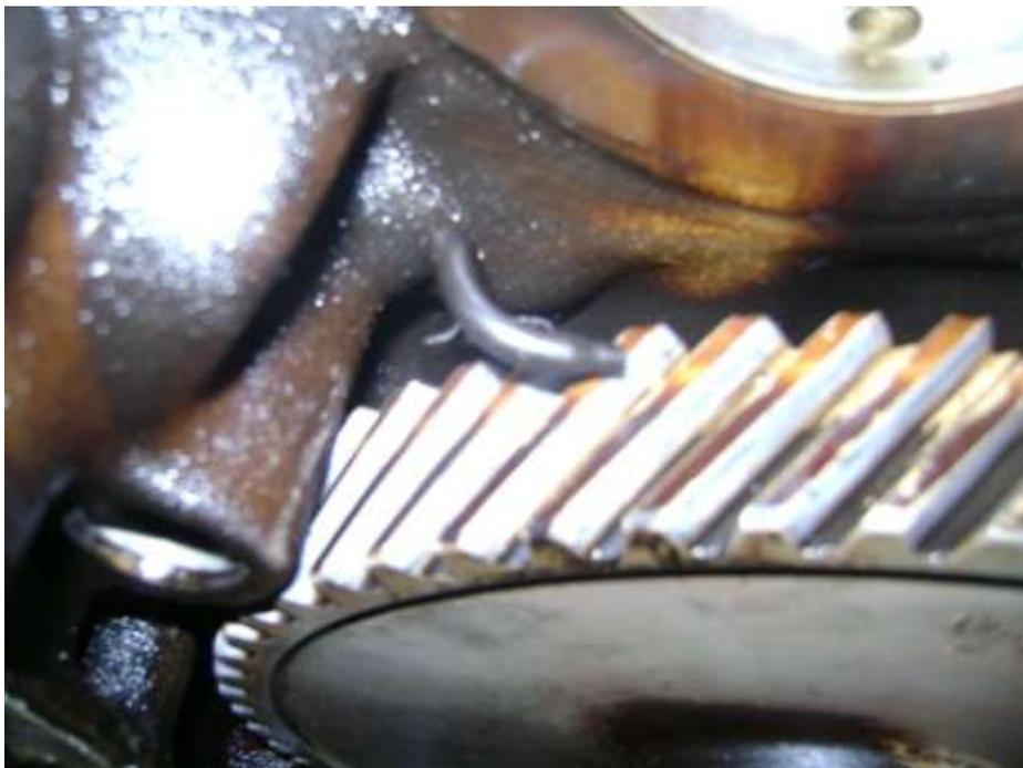
This neat little pipe is fed from the main oil gallery and squirts adequate oil onto the camshaft gear. Note again that the camshaft gear is aluminium driven by a steel gear on the crankshaft. The hole to the left is another view of the oil pump input to the block (the block here is upside down).
