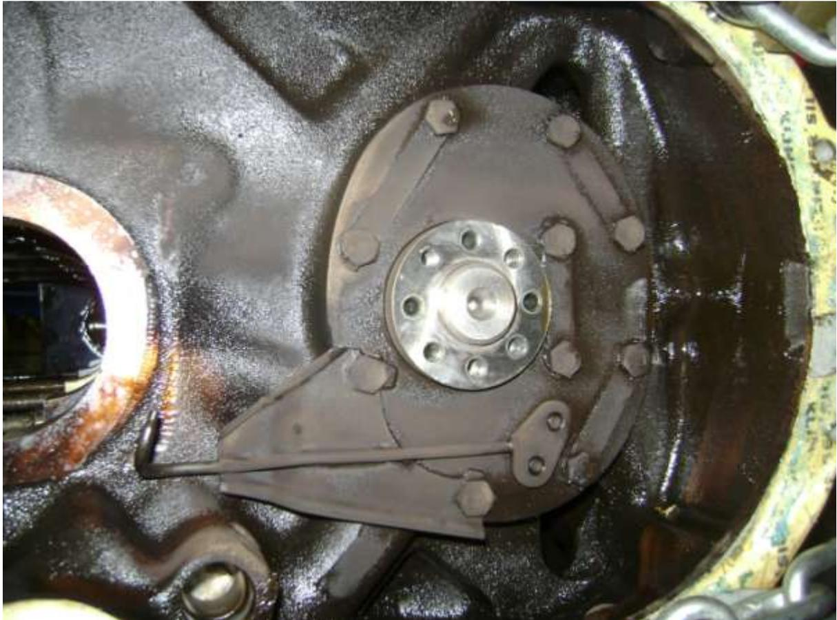
Here is the camshaft thrust plate and cover for the two main oil galleries. The small pipe jet for the camshaft gears is part of the assembly. Below, the camshaft gear has been removed and the camshaft is ready for extraction. The recess surrounding the gear ends in two holes. These are the ends of the main oil galleries that feed the main bearings and thence the big ends.
