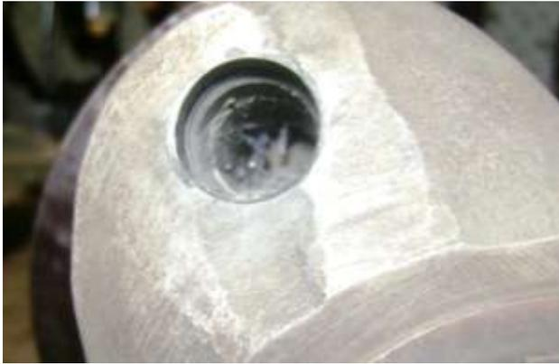
Here is a sludge trap opened which requires a pair of contracting needle nose circlip removers and a small bolt to act as a puller. At lower left this is typical of what you will find. The main pressure oil comes down from the main two galleries that run the length of the block then through drilling to the saddles that the main bearings sit in, through the bearing shells and through the holes drilled in the crankshaft journals. These go direct to the
