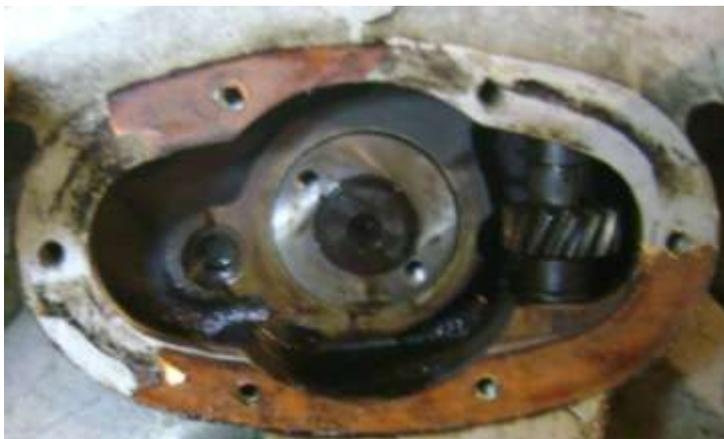
Here the distributor drive gear has been removed exposing the rearmost bearing of the cam shaft. Note that the shaft actually runs in the block and does not have separate bearings. To the left of the shaft is one of two Welch plugs blanking off the rear of the two main oil galleries that run the length of the engine. The other one is behind the distributor gear.
