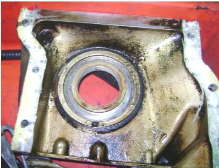
By now all the induction gear is off the top of the engine and the front crankshaft pulleys and bits have been removed. The lower half of the timing case has been removed and inverted for your inspection. In the top left hand dirty corner is a rubber plug. This ingenious bit pushes the oil pump delivery pipe into the gallery leading to the oil filter and then to the big time stuff. If you leave that plug out a lot of
