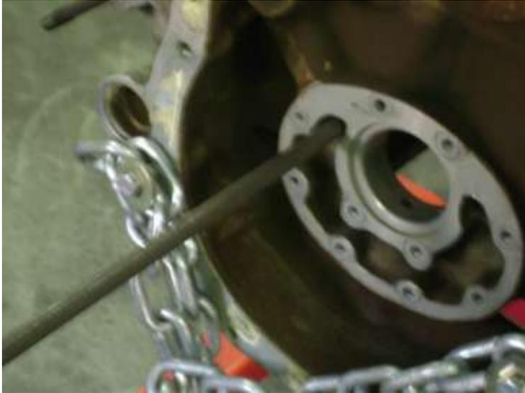
At left poking the Welch plugs out at the other end of the block with a steel rod. This enables the galleries to be thoroughly cleaned particularly after machining. The picture below is taken at the other end showing the brush as it emerged from what was purported to be a clean engine!
