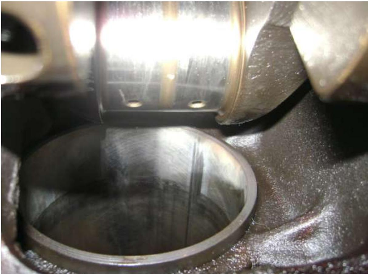
This is view of the bottom end of the liner where it pokes through the bottom of the block. The liner is actually slightly larger than the hole so grips it somewhat tightly and explains why the block needs to be heated to get the things out safely. When the engine is hot the fit must be not quite so tight because if the lower of the two seals at the bottom of the liner has had it, oil from the whirling crankshaft will find its way through the gap and leak out of the weep hole!
