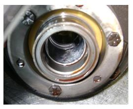
Above. The torque converter normally bolted to the 'flywheel' is a sealed unit (by welding). If you get nasties in the sump and either overhaul the box yourself or have it done, be sure to have the unit opened, flushed and repaired since it is impossible to get muck out of it. It follows that you should also ensure that the transmission oil cooler is flushed.
