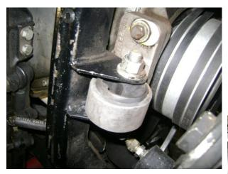
Here you can note the distance between the top of the fan blade and the cowling. Adverting back to the top pic, the rubber insert is shaped to keep the cross bolt nice and high in the holder. In practice the whole thing manages to rotate and lower the engine. A solution to this problem is to install a standard
