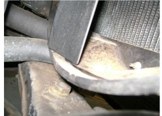
Here note the almost nil clearance between the fan and cowling at the bottom. The location of the engine in post55 vehicles has always intrigued me. The rear mounts of the vee eight are adjustable (at least vertically) and the front mount sometimes has and sometimes hasn't an extra spacer or two to lift the front of the engine. But I have yet to see any guide as to where the engine should actually sit!
