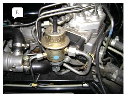
The central bit 'E' here is the fuel pressure regulator. If you are not familiar with fuel injection it comes as a shock to find that the system runs at pressures in excess of 85 psi! This compares alarmingly with the old SU pumps and the Pierburgs running at a pound and a bit! The fuel system is of course recirculating and this little gadget makes sure that the main working bit, the Fuel distributor seen behind the regulator has a constant correct pressure.
