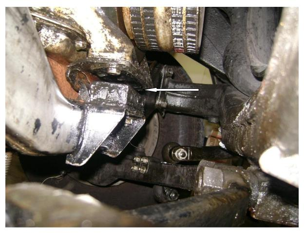
The front end of our cars' engines are notoriously incontinent. This is due to a quaint sealing arrangement between the two castings that close off the front of the engine. The sealing material used hardens and shrinks and oil escapes – all over the front mount. If circumstances prevent correction of this leak and the mount is replaced, wrap it in stout plastic for protection. In the above example the engine has been cleaned albeit too late – the damage has been done.
