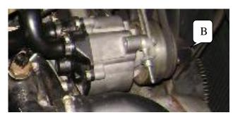
The Air Pump. 'B' This is a gadget spawned by those people who object to being choked by automotive emissions. They have been on the Shadows for years particularly for those cars delivered to the West Coast of America. Given the speed that the engine has to suck in a mixture of fuel and air, set fire to it and get rid of
