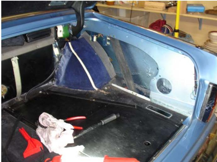
nitrogen of course is trapped or should be in the 'gas springs' screwed into the top of the dampers. If you pull the lining of the boot out you will find them nestled away in the corners above the rear wheel arches.
