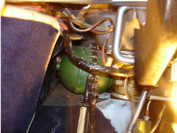
system the car will need to be standing on its wheels. Exhausting the system will let the car sink to a very low level so don't lie underneath while letting the pressure go otherwise you will probably remain there for the rest of your life! You can jack the car up and stand the rear wheels on car ramps or large blocks of wood. Post '86 cars tied both sides of the system together on the one circuit so one bleed screw will empty the lot!
