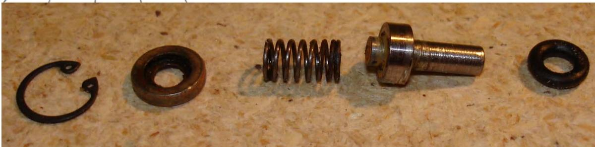
'O' ring threaded over the shank. This is dropped into the hole followed by the normal spring, retainer and circlip and the rubber 'O' ring is jammed between the plunger flange and the seating in the accumulator body.
