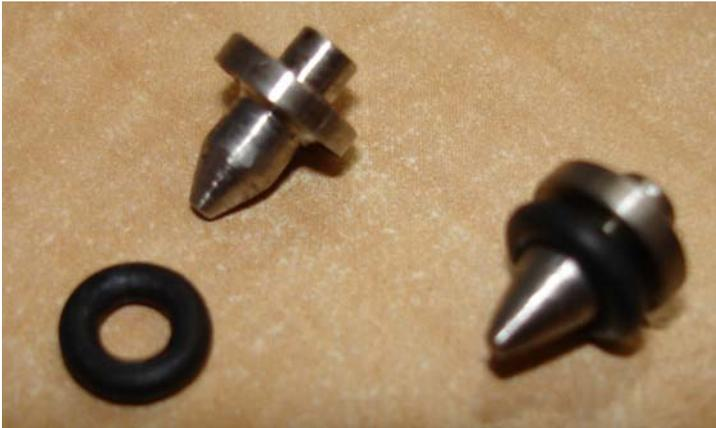
At left is an improvement on the above arrangement in that the tapered tip facilitates the valves entry into the seat. Some operators have found that the seat has been bashed so hard that it was actually distorted the charging hole and the valve has difficulty fitting into it. This of course can be cleaned out by the judicious use of a drill.
