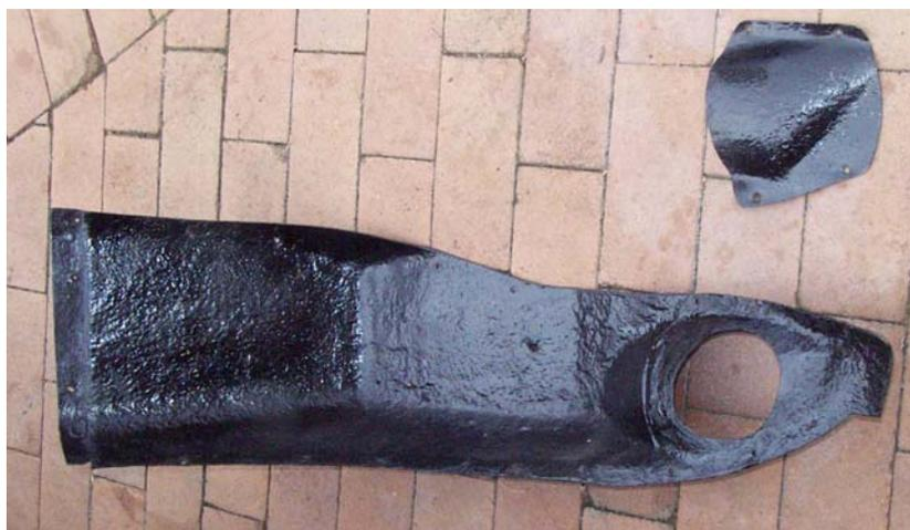
right wheel and then the stone guard gave ready access to the defunct unit. Alas, it also gave ready access superficial rust on the outer panel and a considerable amount of dirt and small stones. So out came the vacuum to do its part. I then applied rust converter to good effect, followed by my favourite POR 15.
