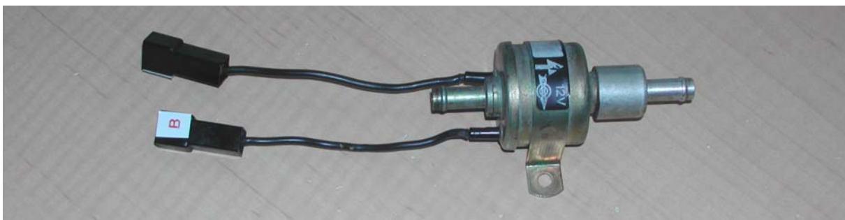
The valve removed. The one mounted adjacent to it is the mixture weakening valve and whilst similar in appearance actually works in the opposite way The above valve is open with the power OFF the other is open when the power is ON.
