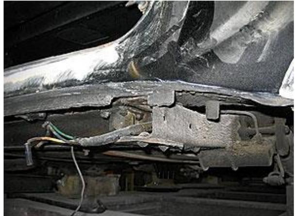
Body sitting on chassis at rear because body mount has collapsed
