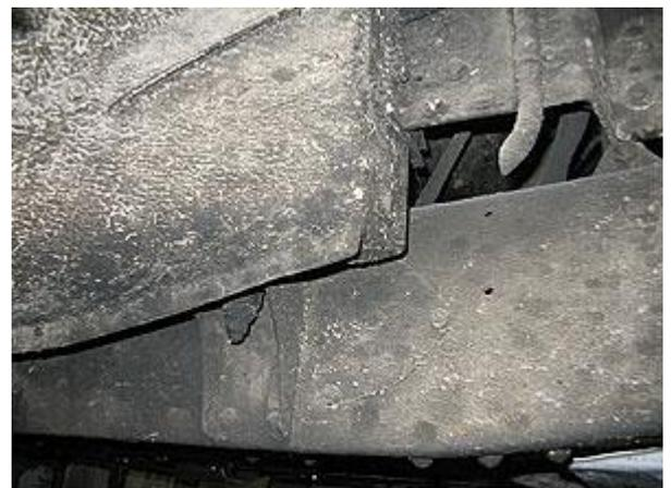
Front end of sill under front wheel arch should be checked thoroughly for rust.
