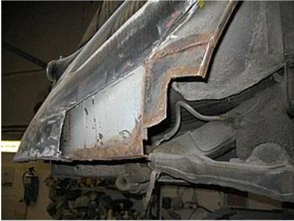
Rear wing in the process of repair
