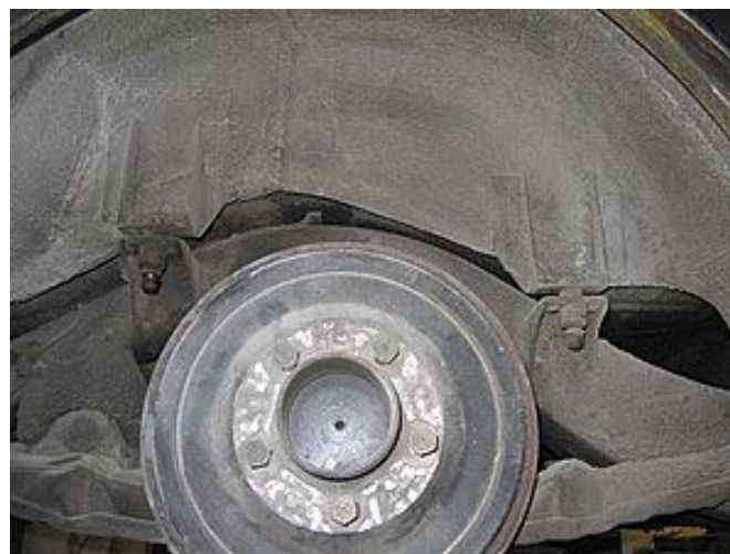
View of inner rear wheel arch showing body mounts, this area can rust leaving body unsupported except at rear.
