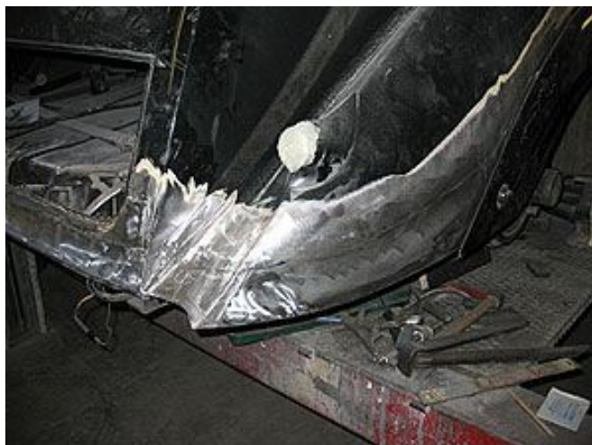
Offside rear wing and lower panel repaired ready for filling and painting.
