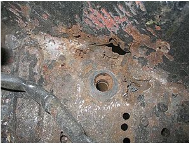
Boot floor around rear body mount needs welding
