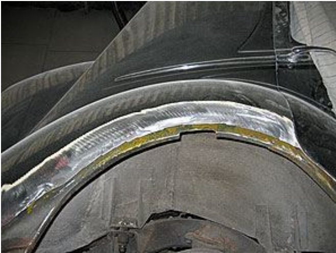
New outer wheel arch flange to be made
