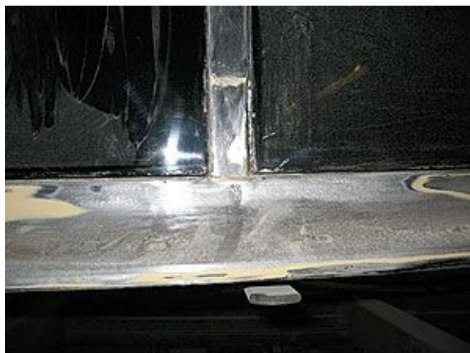
Lower part of B post has had new section welded in
