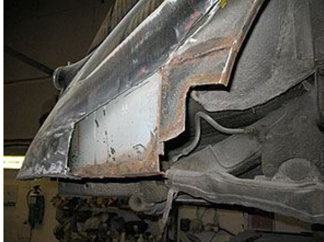
Rear wing in the process of repair
